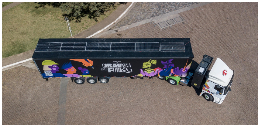
Solar panels on the top of the box. Photos: Paulo Pereira/Teia Documenta
