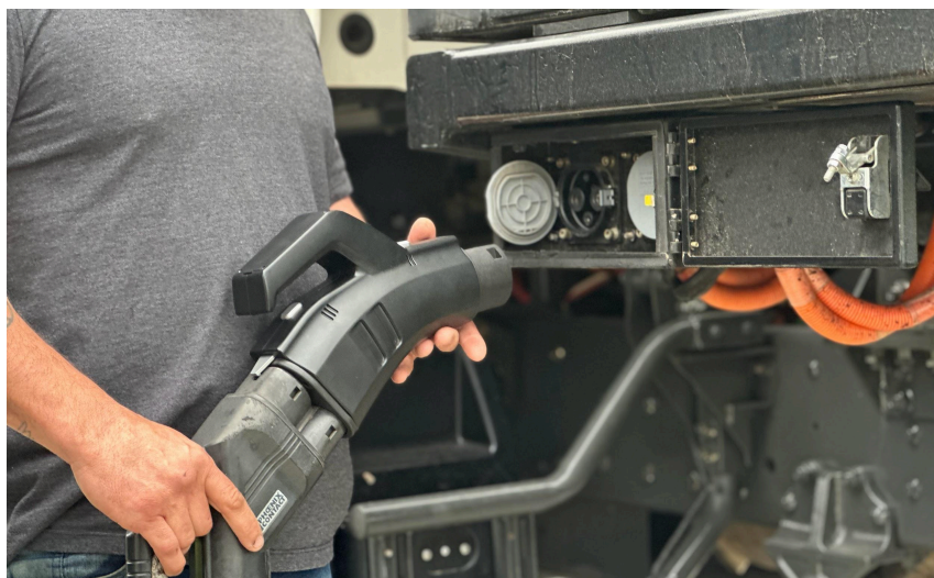
Pair of fast-charging connectors in direct current (DC) according to the GB/T standard, from our truck. Photo: Doug Souza / Quinze Vinte
